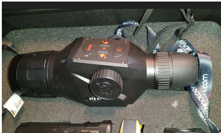
Figure 9. Thermal camera model OTS-4T Thermal Imaging Camera. 640 X 480 Sensor, 40X magnification.
